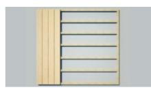
Joists must be installed no further apart than the recommended centres, and there must also be a joist at both ends of the deck board.
