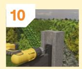
Use two supplied screws to fix each stopper into place.
