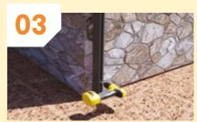
Use the supplied screws to fix the post to the wall, taking care to not over-tighten.
