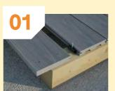
Always use the recommended hidden fixing clips. At the end of the run, an Urban edge board can be used. Fix using a hidden fixing clip and don't over tighten then face fix this board only, using the colour coded screws.
