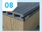
The starter clip is also used as a finishing clip. Install the starter clip to the end of the last joint, slide the deck board between the last clip and the finishing clip.
