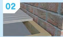
10mm between the wall and deck board.
