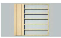
Joists must be installed no further apart than the recommended centres, and there must also be a joist at both ends of the deck board.
