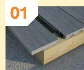
Always use the recommended hidden fixing clips. At the end of the run, an Urban edge board can be used. Fix using a hidden fixing clip and don't over tighten then face fix this board only, using the colour coded screws.
