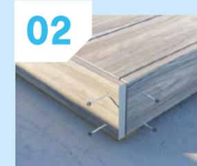
Fix the Habitat+ skirt trim the over Habitat+ deck board edges at the joist ends. Leave a 50mm gap between ground and the trim to aid airflow.
