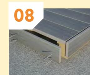
Fix Urban skirt trim underneath the Urban edge board at the joist ends using pilot holes as before. Leave a 50mm gap between ground and the Urban skirt trim to aid airflow. Use two colour coded screws at every joist.
