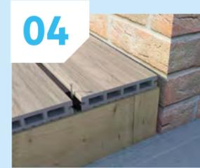
Slide the next deck board into position, locating the hidden fixing clip into its groove. This will set the gap between each deck board. Tighten the hidden fixing clip - but do not over tighten, use a low speed high torque setting on your electric screwdriver. Duplicate this step for every additional board.
