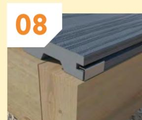
The starter clip can also be used as a finishing clip. Install the starter clip to the end of the last joint, slide the deck board between the last clip and the finishing clip.
