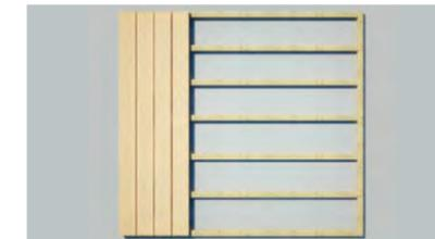
Joists must be installed no further apart than the recommended centres, and there must also be a joist at both ends of the deck board.
