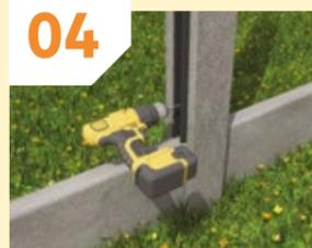
04 Starting at the bottom, fix the fence post connector to the concrete post with the supplied screws. Don't over-tighten.
