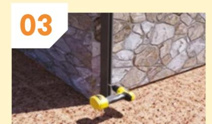
**03** Use the supplied screws to fix the post to the wall, taking care to not over-tighten.
