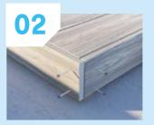
Fix the Habitat+ skirt trim the over Habitat+ deck board edges at the joist ends. Leave a 50mm gap between ground and the trim to aid airflow.
