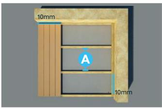
Choose the decking design required, whether it is vertical, horizontal or the herringbone/chevron design. A min of 50mm free air space must be available between the bottom of the deck boards and the ground surface.
