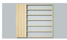
Each board should be supported by 3 joists. Ensure a slight fall of 2° to aid water run off.
