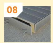
Fix Urban skirt trim underneath the Urban edge board at the joist ends. Leave a 50mm gap between ground and the Urban skirt trim to aid airflow. Use two colour matched screws at every joist.
